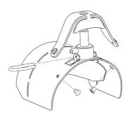
Figure 4. **Brace removal** Remove Allen key fixings. Lift upwards for removal
